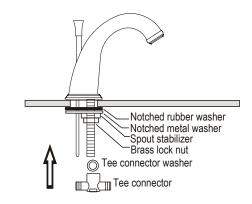
2 - Slip the spout mounting hardware back onto the spout. First the notched rubber washer, then the notched metal washer and lastly the brass lock nut. Hand tighten the lock nut.
